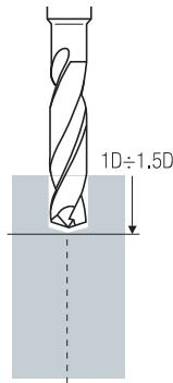
MACHINING OF DEEP HOLES PERPENDICULAR TO THE SURFACE
